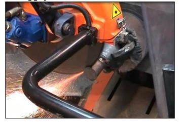
**Cutting Aluminium with abrasive wheel**
