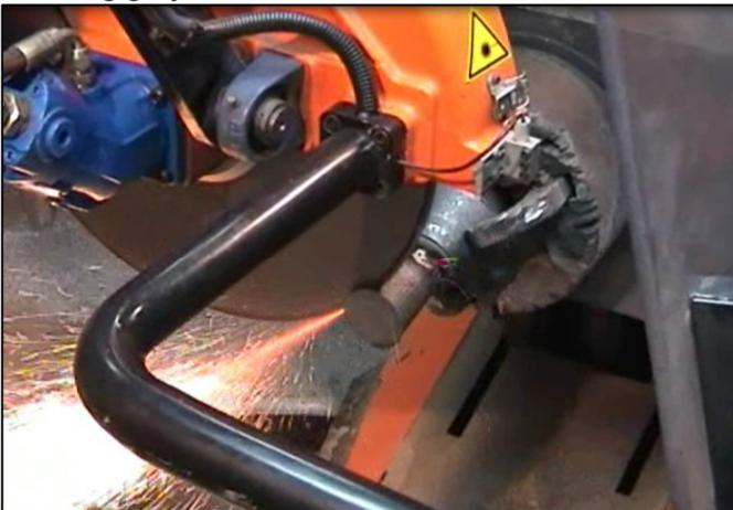
Cutting Aluminium with abrasive wheel
