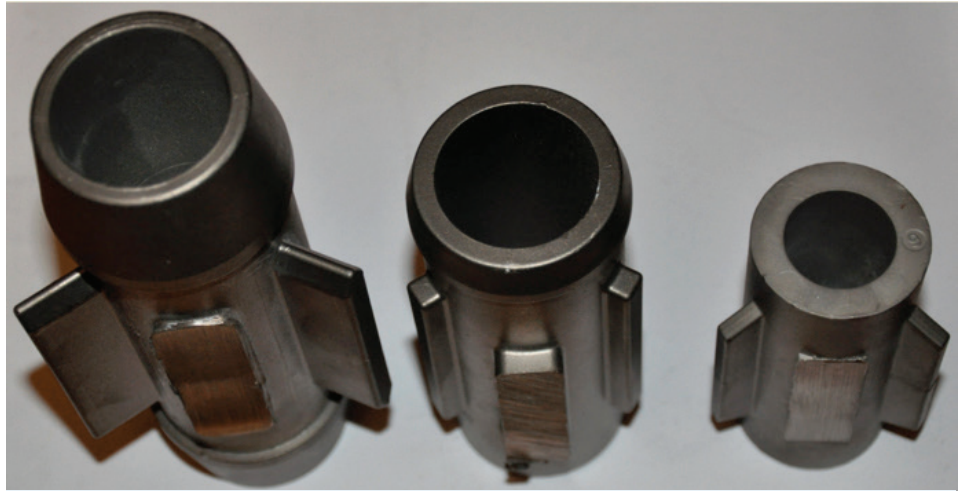
Figure 1: Part Family after Initial Plunge Grind
