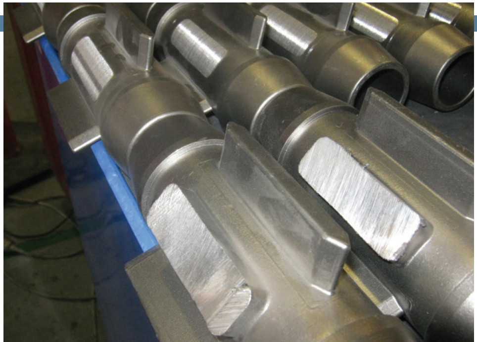
Figure 6: Parts before grind (foreground) and after (above) Figure 7 & 8: CAD & Finished Product Comparison (below)
